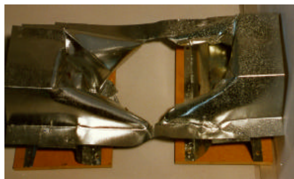
Fig.7 Trapezoidal steel sheet after the experiment. Arc length under water: 2x12cm. Impulse Current : 10/350μs; Peak= 49,6 kA; Char-
