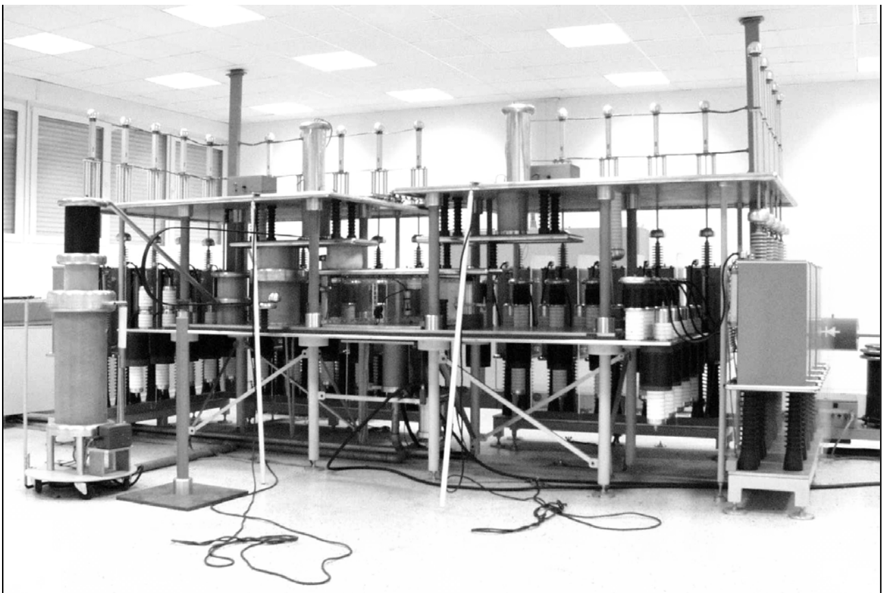
Fig. 2: Surge current generator of the BET
