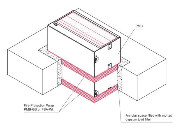
The Fire Protection Wrap PMB-GS or FBA-WI must be fixed to Fire Protection Box PMB so that it is flush with the surface of the floor on both sides.
