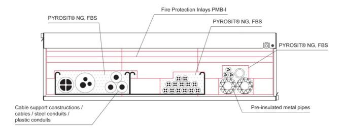
All joints and gaps between the penetrating elements and between the penetrating elements and PMB resp. PMB-I have to be filled with PYROSIT® NG, FBS.
