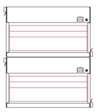
Two Fire Protection Boxes PMB may be stacked. The Fire Protection Wrap PMB-GS or FBA-WI has to be fixed around each fire protection box in accordance with ANNEX B.1 and B.2 of the ETA.
