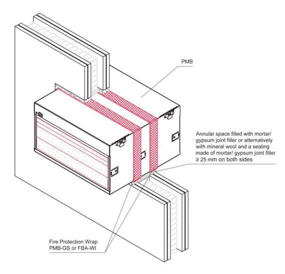
The Fire Protection Wrap PMB-GS or FBA-WI must be fixed to Fire Protection Box PMB so that it is flush with the surface of the wall on both sides.
